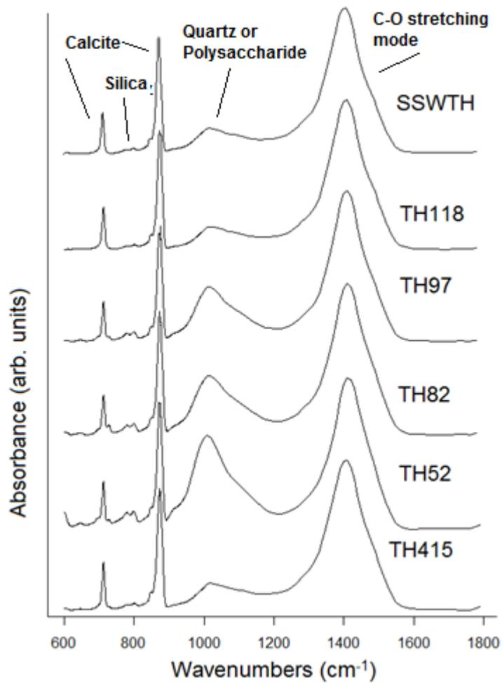
Figure 4: Representative spectra of FTIR results for samples from locality 2, peak allocations are labelled in figure.
