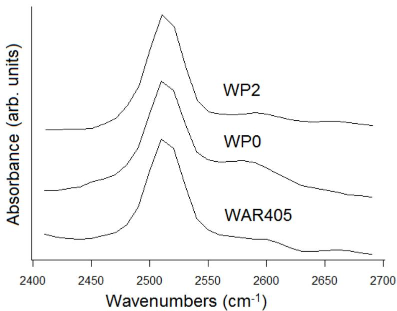
Figure 5: Representative spectra showing a dolomite peak at  $2511\text{cm}^{-1}$
